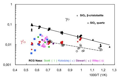
Figure 10: Comparison of our experimental results of  $\gamma$  (on  $\beta$ -cristobalite and quartz, in black) and  $\gamma$ ' (on  $\beta$ -cristobalite, in red) with those of RCG Nasa from [1, 3-5] versus reciprocal temperature
