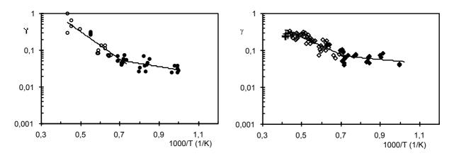
Figure 6: Atomic oxygen recombination coefficient  $\gamma$  for two sintered alumina samples versus reciprocal temperature: A on the left and B on the right
