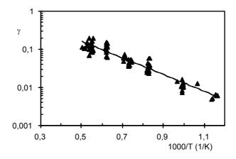
Figure 7: Atomic oxygen recombination coefficient  $\gamma$  for alumina on AIN versus reciprocal temperature
