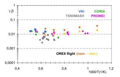
Figure 12: Comparison of the effective recombination coefficient γ' for OREX materials versus reciprocal temperature
