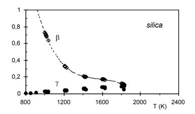
Figure 8:  $\gamma$  and  $\beta$  recombination coefficients versus temperature for cristobalite (silica)
