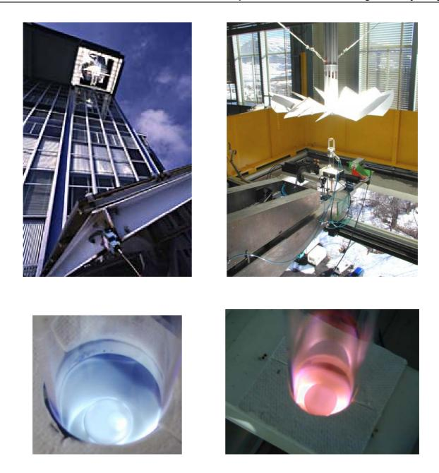
Figure 1: Experimental set-up MESOX with the irradiated shutter (top, right) placed at the focus of the 6 kW solar furnace (top, left). Images of plasma environment: CO<sub>2</sub> (down, left) and air (down, right).
