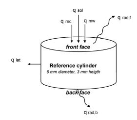
Figure 2: Reference cylinder considered for the evaluation of the thermal flux of recombination under air plasma conditions
