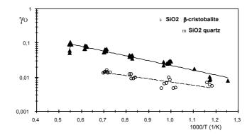
Figure 4: Atomic oxygen recombination coefficient  $\gamma$  for SiO<sub>2</sub>  $\beta$ -cristobalite and quartz versus reciprocal temperature
